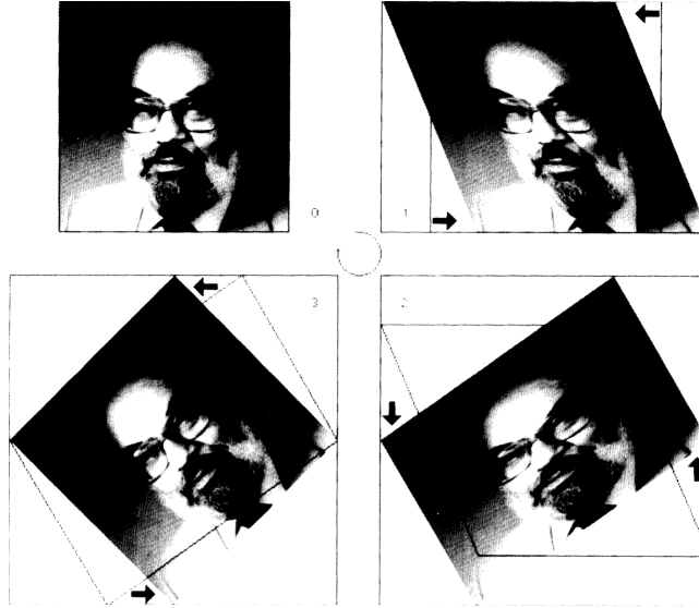
Figure 3. Rotation of an image is carried out by cascading translation operations, courtesy of Unser et al. [9].
